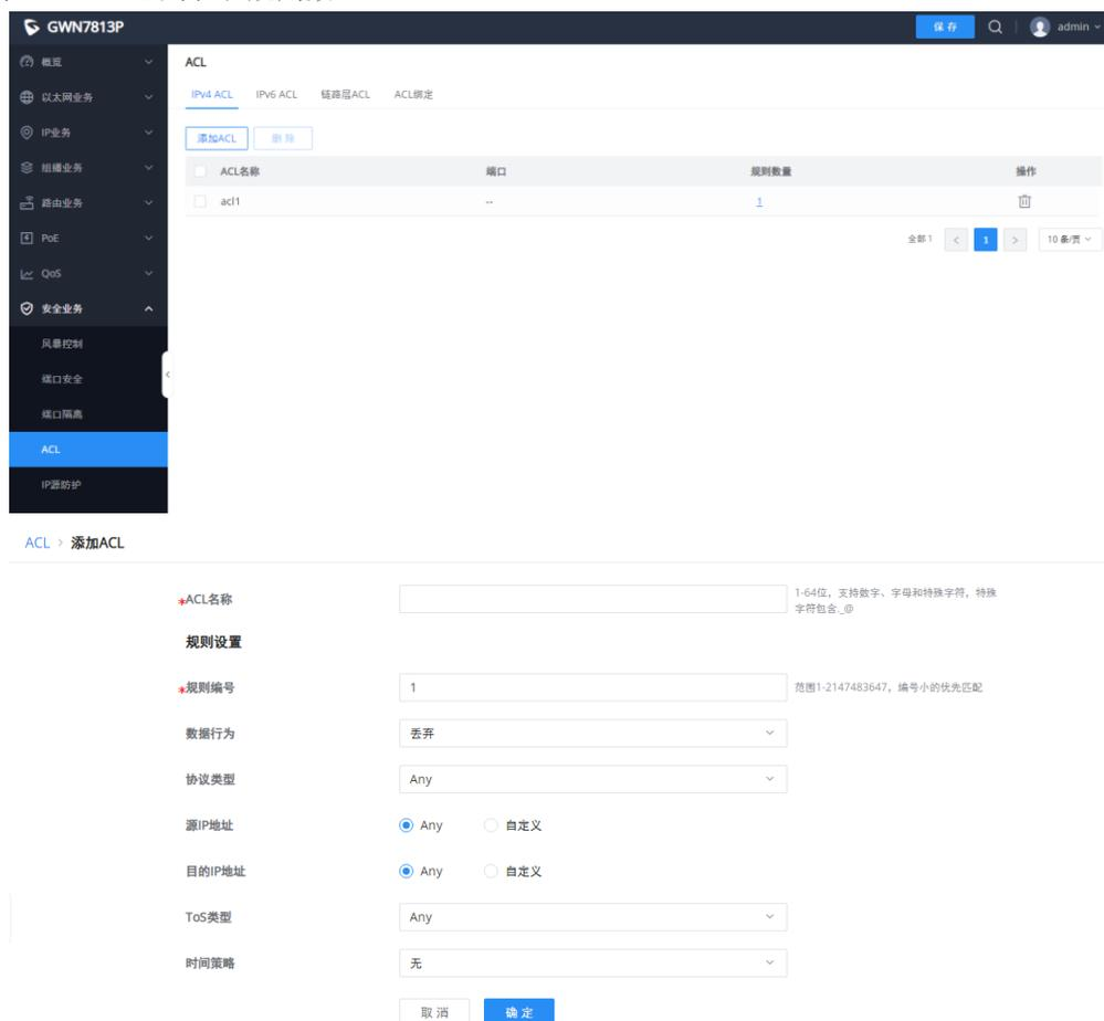
The screenshot displays the web management interface for a GWN7813P device. The main menu on the left includes sections like 'Overview', 'Network Services', 'IP Services', 'Routing Services', 'PoE', 'QoS', and 'Security Services'. The 'Security Services' section is expanded to show 'ACL', 'Port Security', and 'Port Isolation'. The 'ACL' page is active, showing a table of IPv4 ACL rules. Below the table is a form to add a new ACL rule.
