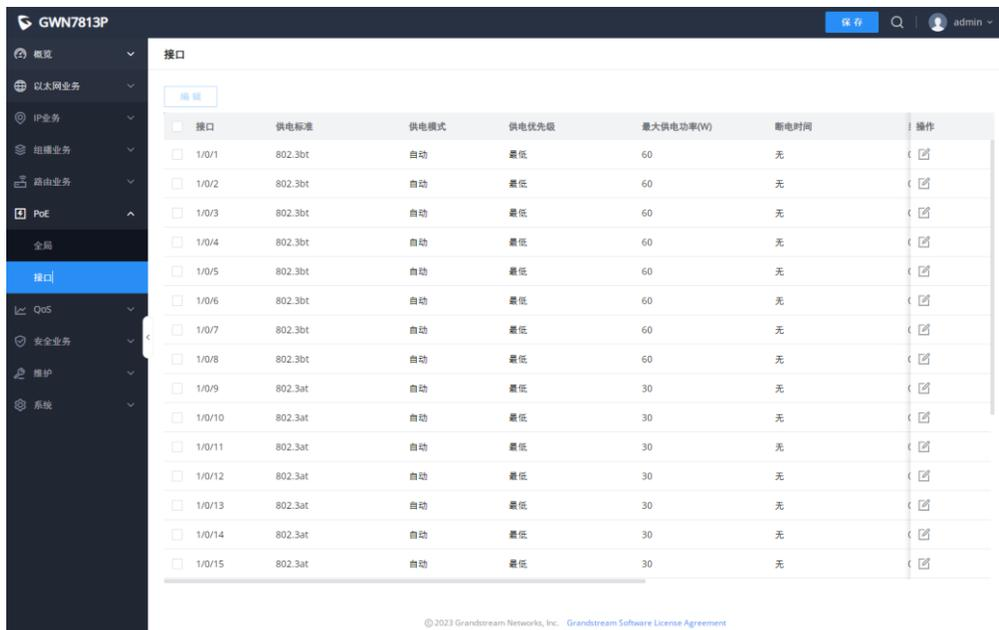
The screenshot shows the configuration page for PoE on a GWN7813P switch. The interface includes a sidebar menu with options like 'Overview', 'Ethernet Services', 'IP Services', 'VLAN Services', 'PoE', 'Global', 'QoS', 'Security Services', 'Maintenance', and 'System'. The 'PoE' section is expanded to show the 'Interface' configuration table.
